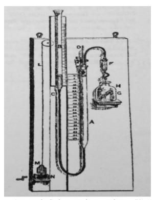
Figure 4. The Carbometer of Pruen and Jones (32).
