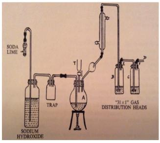
Figure 11. Residual CO, Apparatus (76).
