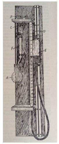
Figure 8. Chittick Apparatus (AOAC 1925, Ref. 54)
