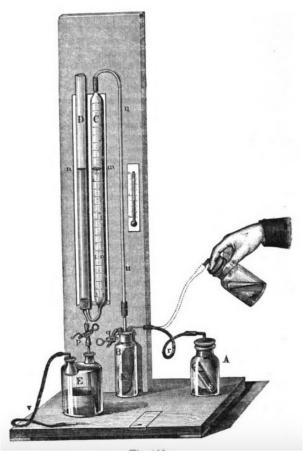
Figure 2. Scheibler's Apparatus from Fresenius (19).
