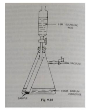
*Figure 9.* Determination of  $CO_2$  under reduced pressure (75).
